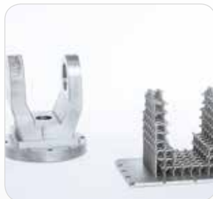
Fork with a supporting structure
